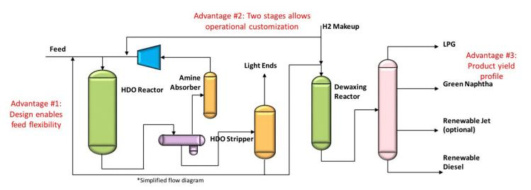
EMRD, ExxonMobil's proprietary process technology
